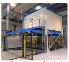
Heat treating furnace - Quenching of aluminum parts – Aeronautics
